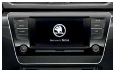
6.5" SWING infotainment unit with Bluetooth and a USB port as standard
